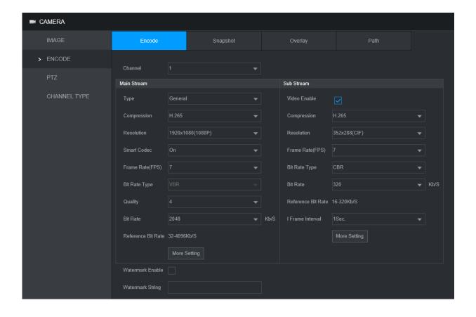
In this menu you can set the compression, resolution frame rate and bitrate etc. for each camera. Note that max. frame rate may be capped differently for certain channels. Resolution should be set automatically when the camera is detected.
